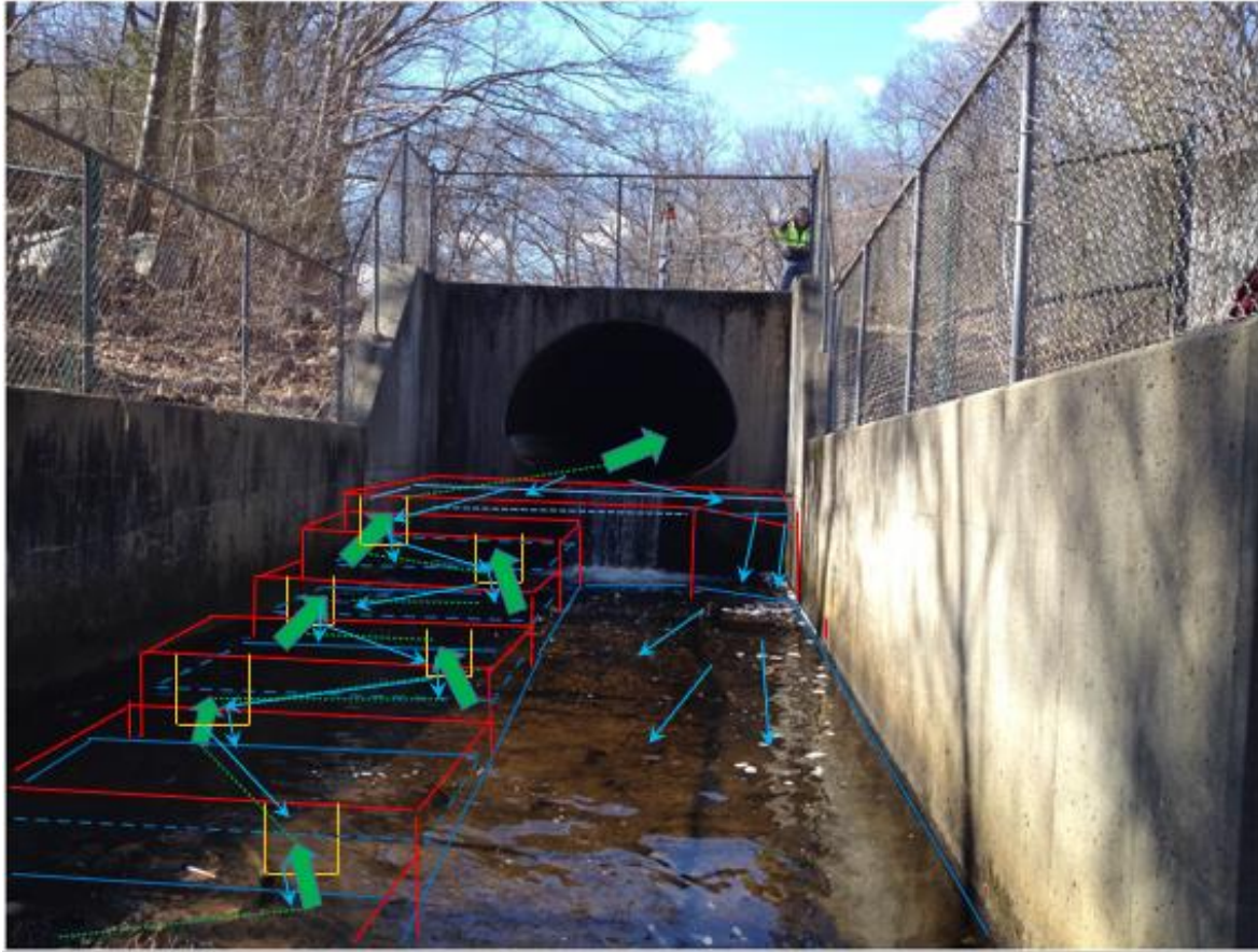
Figure 11-1: Alternative 2 - Fish Ladder on One Side of Stilling Basin, conceptual rendering. Fish passage illustrated in green, streamflow in blue.
